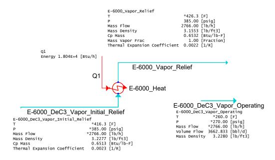
Heat Time = 18,040 Btu / 1,340,000 Btu/hr = 0.0135 hr = 0.81 min Mass Released = (3.2277 lb/ft3 - 3.1553 lb/ft3) \* 857 ft3 = 62.3 lbRequired Rate = 62.3 lb / 0.0135 hr = 4,628 lb/hr
